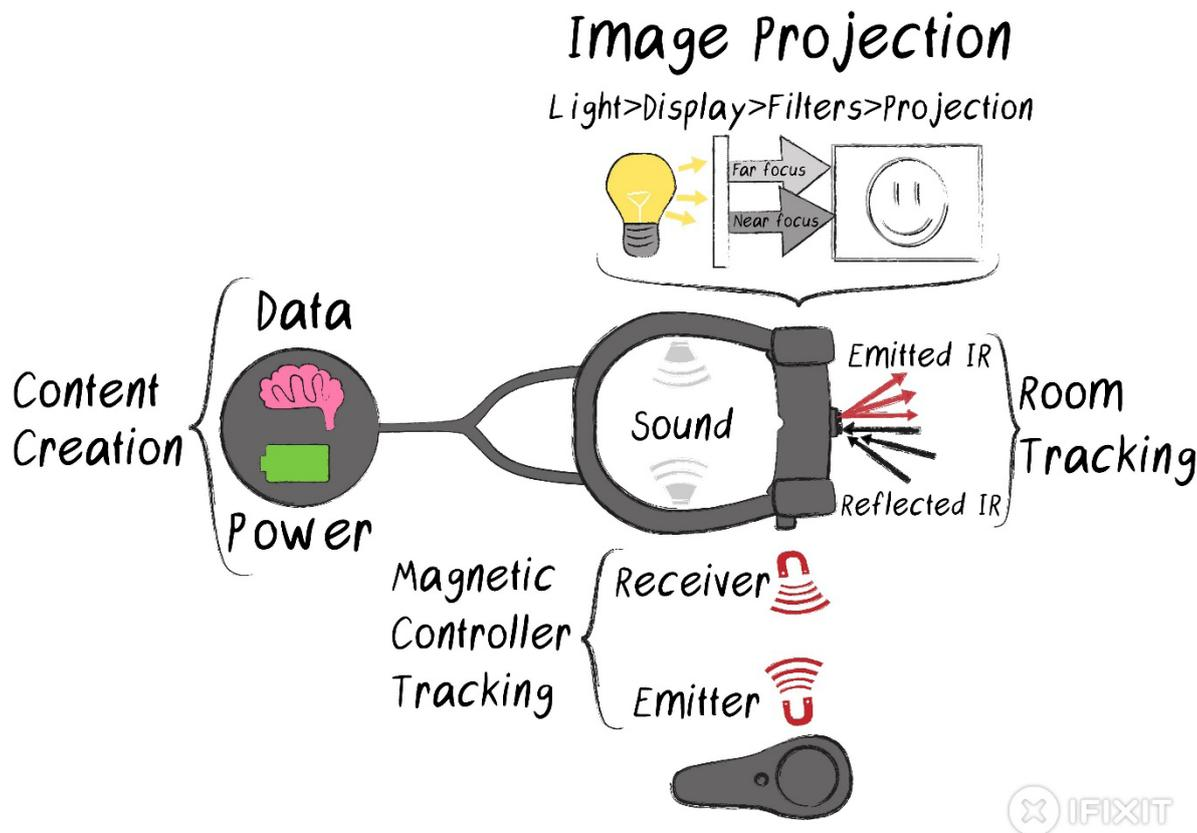
Figure 1: A visualization of how the Magic Leap works (IFixit, 2018).
